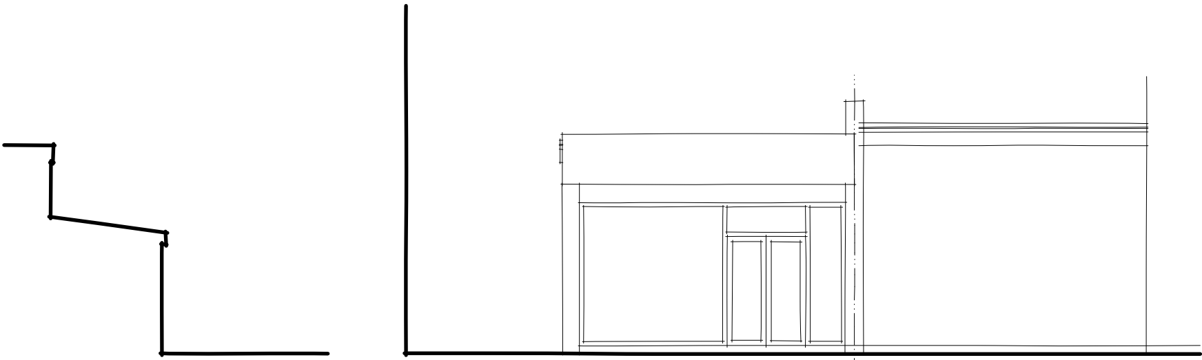
EXISTING FRONT ELEVATION 1:100
